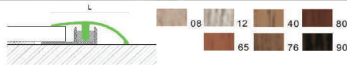
T-LAJSNA ZA RAZLIČITE VISINE ALUMINIJ 40 mm L=270 cm 0994380 ZLATNA C/7/SF ART.67017 0994381 SREBRNA C/7/SF ART.67007 0994382 BOJA DRVETA 12 C/7/SF ART.66009 0994383 BOJA DRVETA 40 C/7/SF ART.66037 0994384 BOJA DRVETA 65 C/7/SF ART.66065 0994385 BOJA DRVETA 76 C/7/SF ART.66074 0994386 BOJA DRVETA 80 C/7/SF ART.66077 0994387 BOJA DRVETA 90 C/7/SF ART.66087
